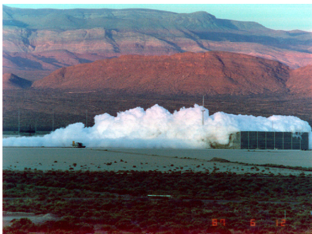
Fig. 13. Falcon 1 spill showing LNG vapor overflowing the vapor fence.
